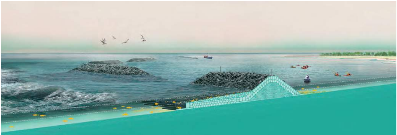
Fig. 7 Section of proposed living breakwater coastal condition. Image courtesy of Scape Studio.
